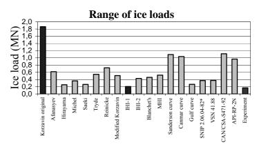
Figure 1. Correlation between ice loads obtained from experiment and value of ice load calculated with different methods
