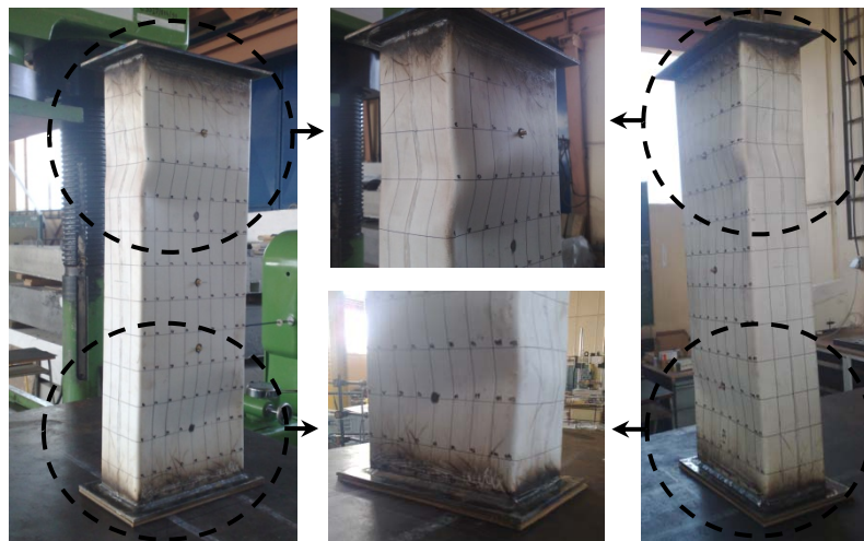
Figure 4. Test completion and overall failure; member B22
