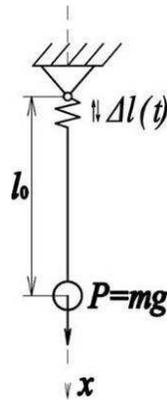
Figure 1.5. Spring pendulum
