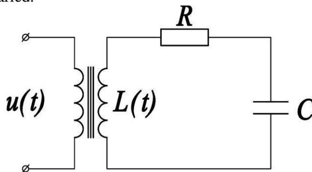
Figure 1.12. Transformer oscillatory circuit
