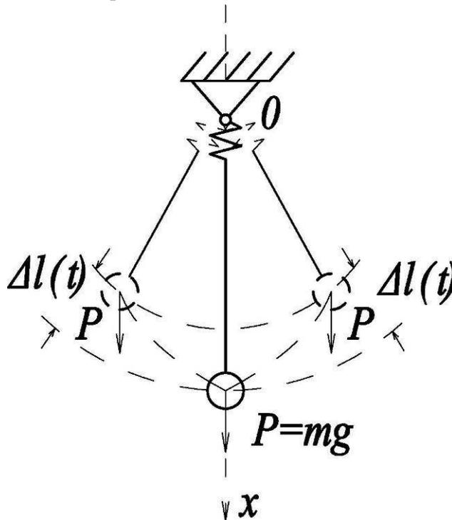
Figure 1.6. Spring pendulum oscillation
