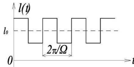
Figure 2.10. Step-wise law of effective pendulum length variation
