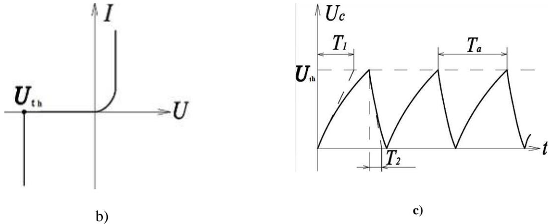
**Figure 1.18. Self-excited capacitor voltage oscillations**
