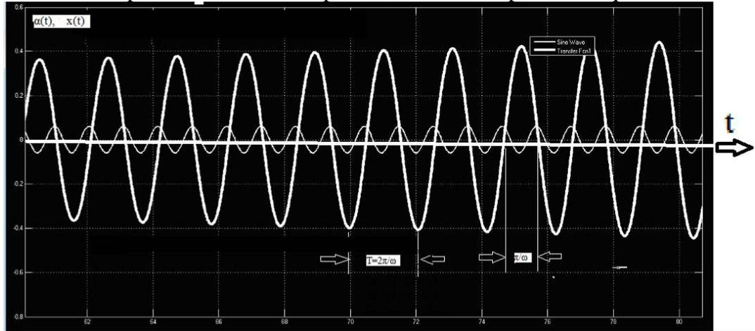
Figure 1.4. Ramp parametric oscillation of pendulum
