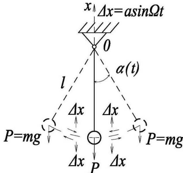
Figure 1.3. Pendulum with suspension point vibration
