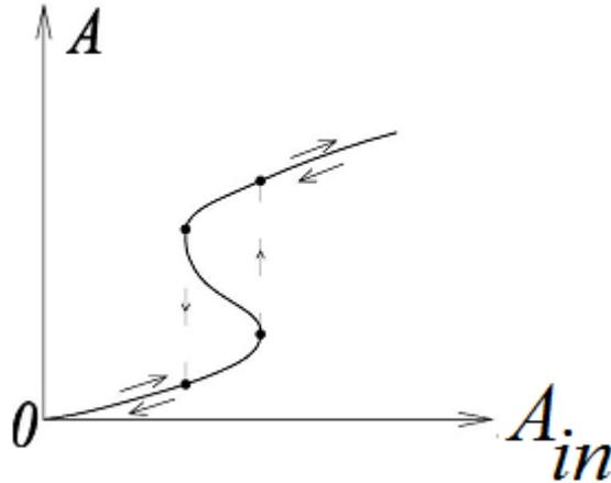
Figure 2.12. Step-wise resonance illustration
