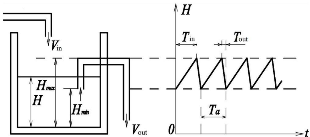
Figure 1.17. Self-excited oscillations of liquid level in Tantalus vessel
