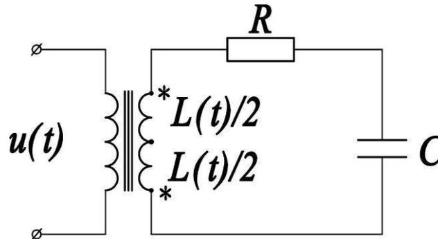
Figure 1.13. Inductive parametric resonance
