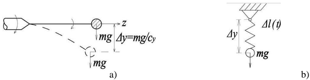
Figure 1.8. Simplified model of elastic shaft oscillation
