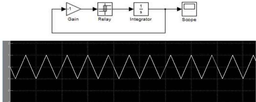
Figure 2.14. Rough model of self-excited system
