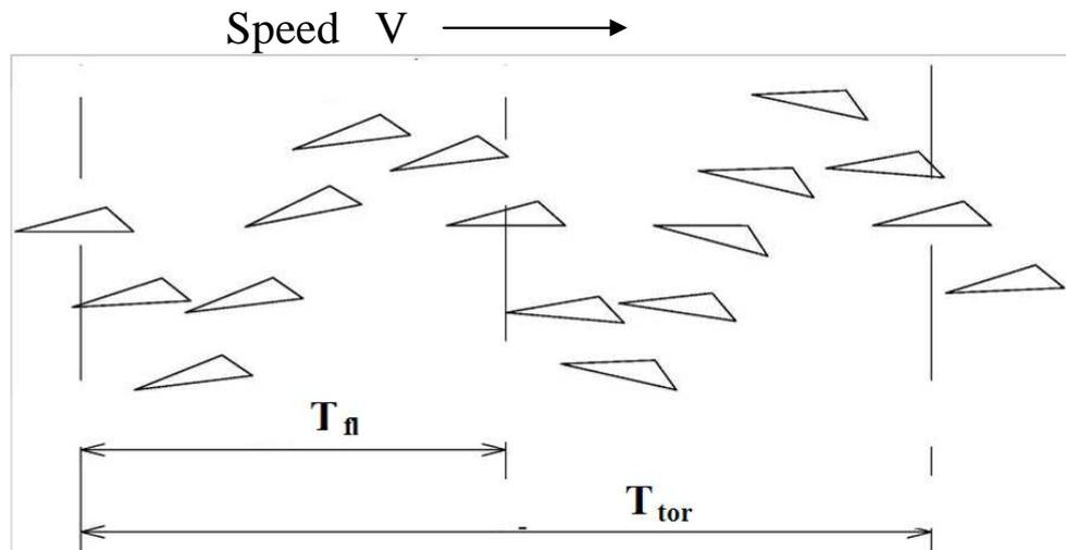
Figure 1.16. Flexure-torsion oscillations
