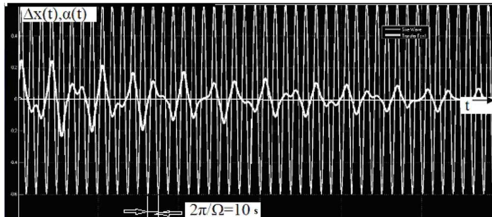
Figure 1.10. Transient of inversed pendulum stabilization
