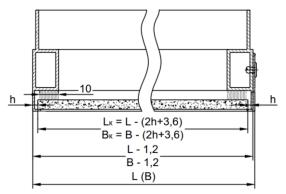
Figure 3. Constructive scheme of facade cassette
