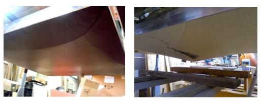
Figure 11. Destruction of cassette under the influence of distributed load
