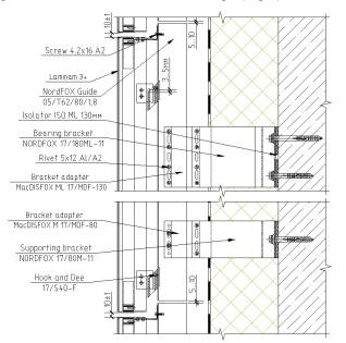
Figure 4. Section of facade system
