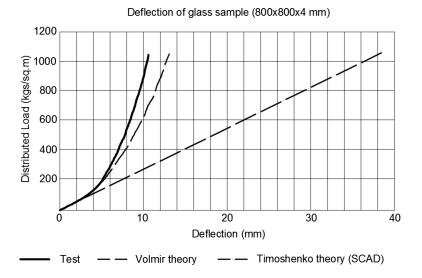
Figure 10. Results of glass plate test
