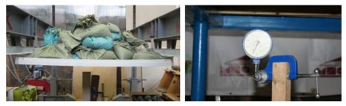
Figure 6. Testing stand (left) and deflectometer 6PAO (right)
