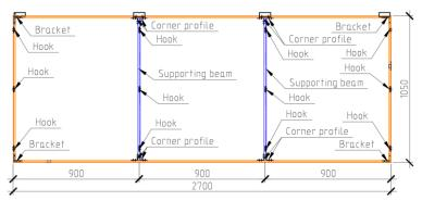
Figure 8. Example of cassette with dimensions 2700x1050 mm
