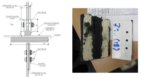
Figure 5. Testing scheme (left) and breaking results (right)
