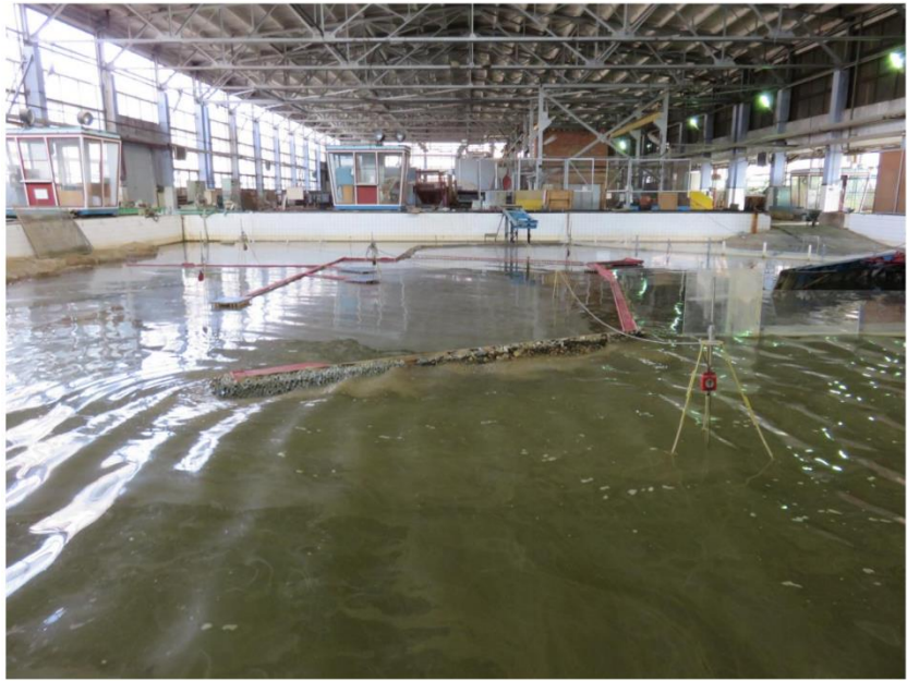
Figure 9. General view of the wave field generated by South Waves during physical modelling
