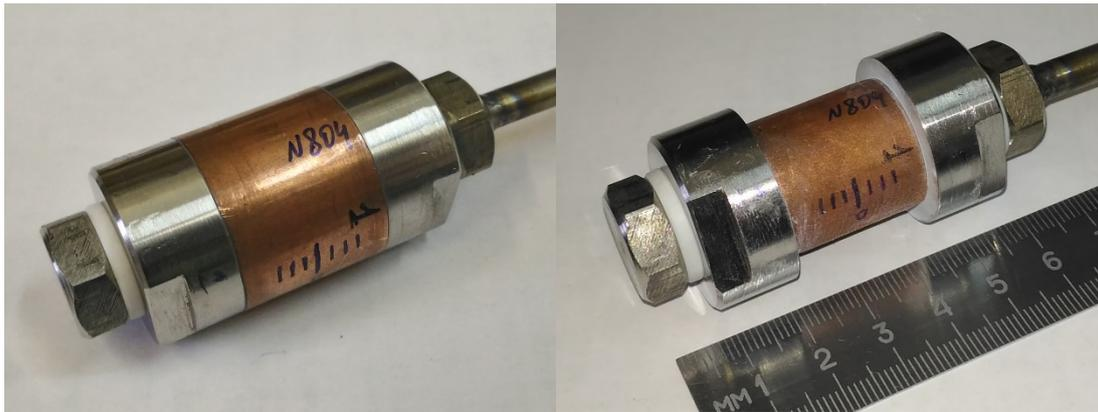
**Fig. 6.** View of fitted mold (sample No. 804) before (left) and after (right) the MPC
