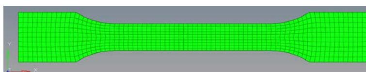
**Fig. 5.** Finite element model of standard specimen.
