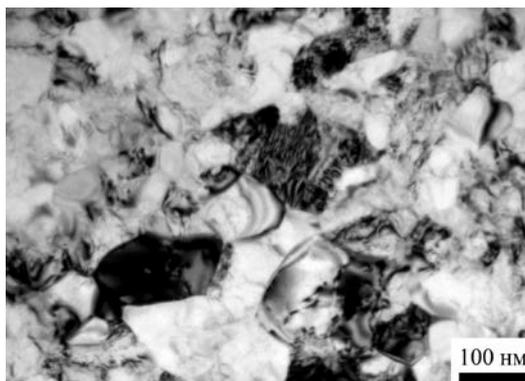
**Fig. 1.** Nanotitanium microstructure.
