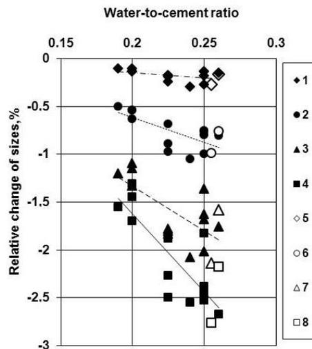
**Figure 7. Water-to-cement ratio dependence of radiation-change of volume of Portland cement stones with and without various superplasticizers additives – after brief (5 hours) heat treatment at various temperatures**
