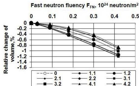
Figure 4. Dependence of calculated radiation change in volume of Portland cement stones with and without various superplasticizers based on polycarboxylated ethers, on fluency of fast neutrons with charge above 0.8 MeV
