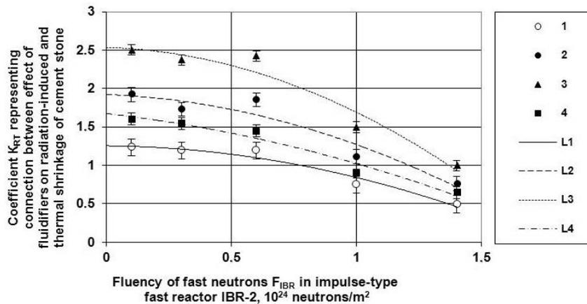
**Fig. 1. Dependence of coefficient  $K_{RT}$  representing the effect of superplasticizers on radiation-induced and thermal change of volume of Portland cement stone, on fluency of fast neutrons in impulse-type fast reactor IBR-2, based on comparison of Portland cement stone exposed to radiation in reactor with same briefly (5 hours) heated at 150, 350, 600 and 900 °C**
