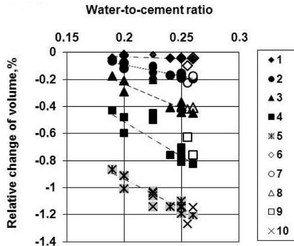
**Figure 6. Water-to-cement ratio dependence of radiation-change of volume of Portland cement stones with and without various superplasticizers additives – after radiation treatment with different fluency of fast neutrons charged above 0.8 MeV**
