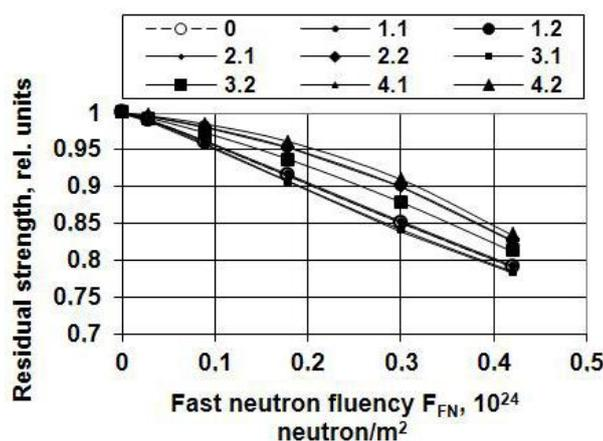
**Figure 5. Dependence of calculated relative residual strength to compression in Portland cement stones with and without various superplasticizers based on polycarboxylated ethers, on fluency of fast neutrons with charge above 0.8 MeV**
