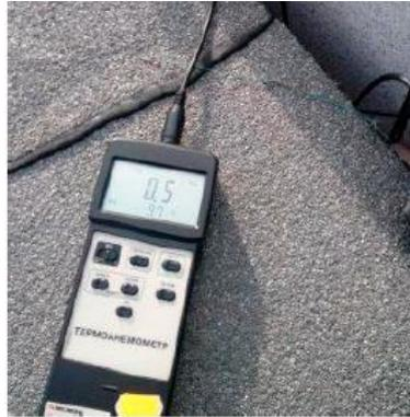
Figure 4. Thermal anemometer
