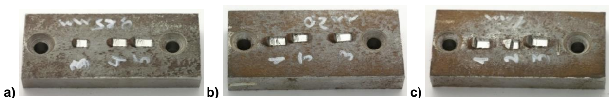
Figure 5. Appearance of specimens after indentation with further shear tests. Initial indentation depth: a) 150 \mu\text{m} , b) 350 \mu\text{m} , c) 750 \mu\text{m}
