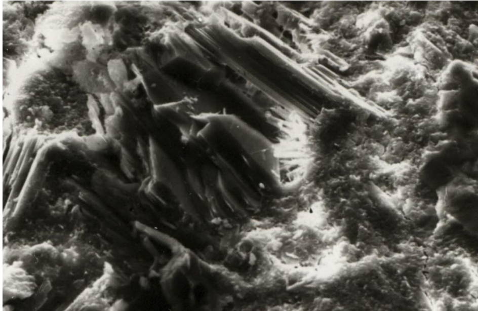
Figure 6. Mixed crystal of hydration products (ettringite, portlandite, hydrosilicate) in the black aggregate volume: zoom x10000
