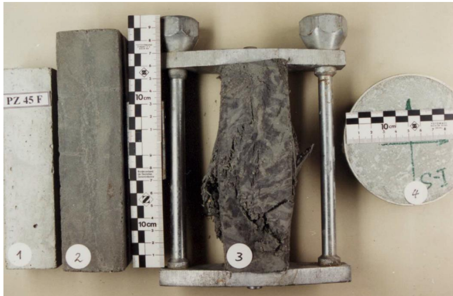
Figure 1. The influence of expansion deformation constraint degree on the change in volume of the expanding concrete of B 35 grade (2 ÷ 4).
