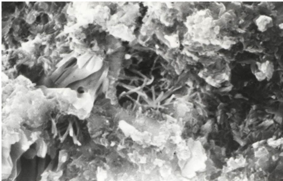
Figure 7. Transition zone between the black agglomerate and gray matrix, zoom x10 000: ettringite, portlandite, silicate hydrate, calcite
