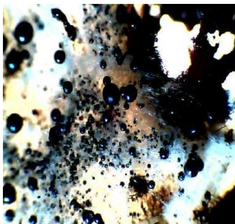
Picture 5. Solidified droplets of metal spatter, 50µm on filter fiber
