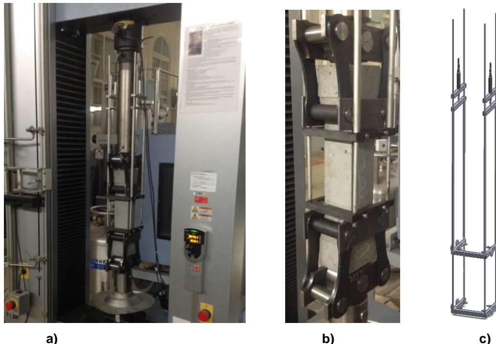
Figure 2. Test machine (a), tensile test fixtures (b) and strain sensor frame (c)
