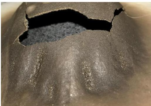
Figure 3. Formed foam with unheated side
