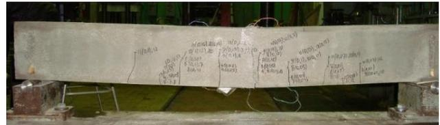
Figure 6c. Typical collapse in models of Group B7
