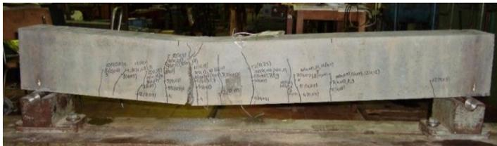
Figure 6b. Typical collapse in models of Group B2
