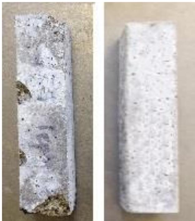
**Figure 1. Samples after the accelerated test on alkali-silicate interaction**
