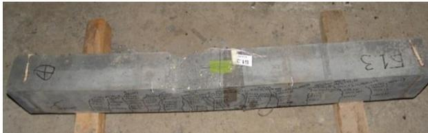
Figure 6a. Typical collapse in models of Group B1
