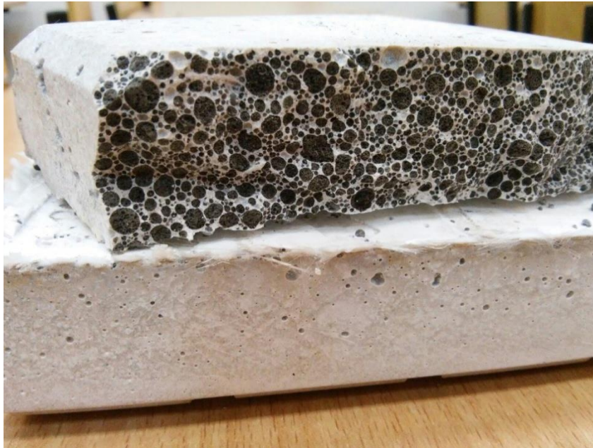
Figure 2. Sample section of lightweight concrete based on the magnesia binder
