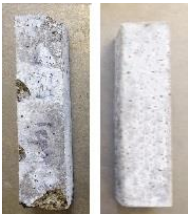
Figure 1. Samples after the accelerated test on alkali-silicate interaction
