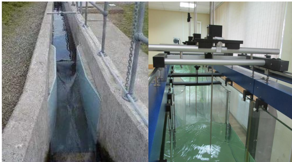
Figure 1. Venturi flumes: on the left – prototype (view from downstream pool); on the right – model (view from upstream pool)
