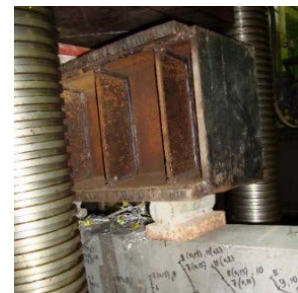
Figure 7. Diagram of load transfer to the models
