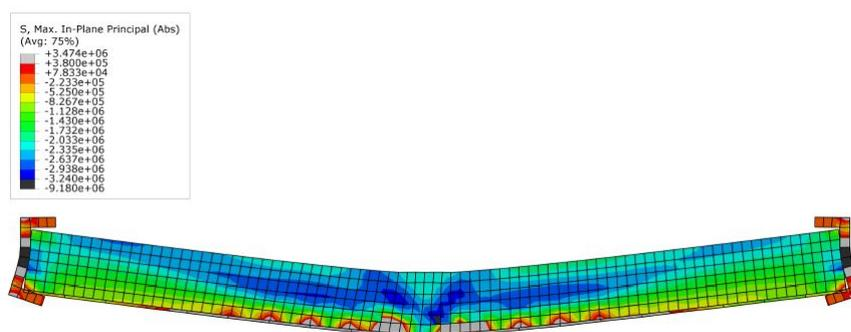
**Figure 6. Stress-strain state of a reinforced specimen under action  $N=120\text{ kN}$  и  $M=1.51\text{ kN}\cdot\text{m}$**
