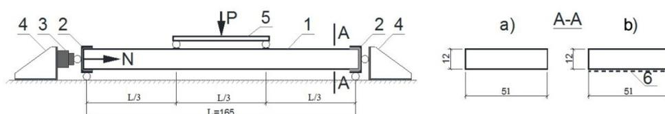
**Figure 2. Scheme of tests of unreinforced (a) and reinforced (b) masonry compression specimens with bending (dimensions in cm)**
