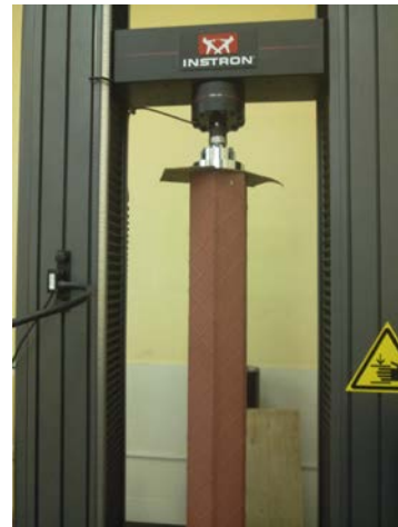
Figure 4. Compression tests of a HWPC sample on Instron 5982 test machine
