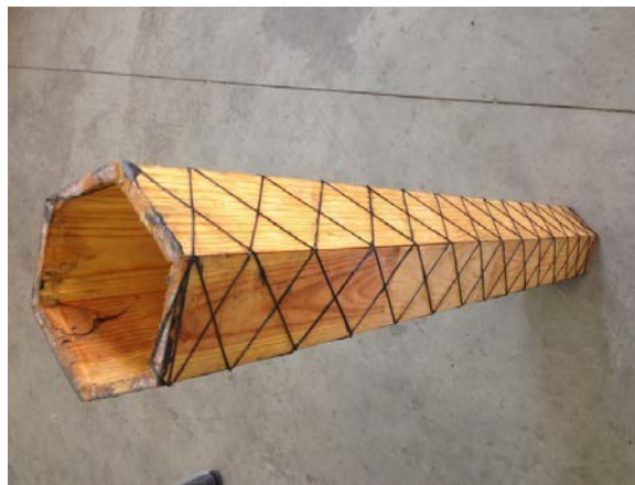
Figure 1. HWPC sample with external reinforcement in the form of a carbon fiber grid
