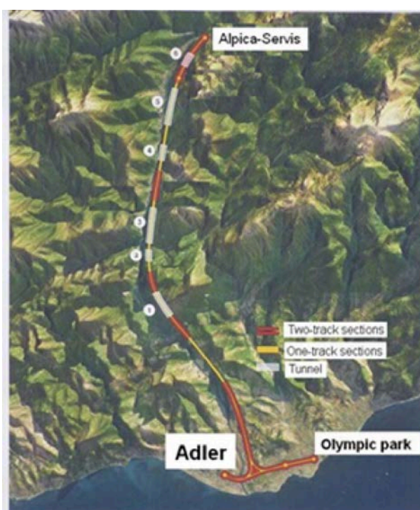
Figure 1. Tunnel routes layout
