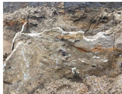
Figure 16. A section of the injected plot after the injection of the resin (The investigated soil and the resin propagation)
