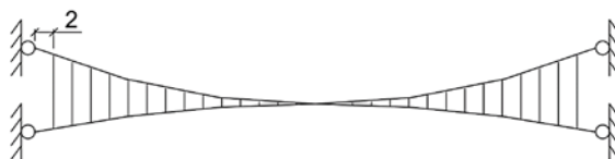
Figure 1. The cable truss with the vertical suspenders and chords joined in the middle of the span [4]
