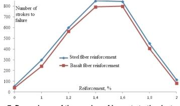
Figure 7. Dependence of the number of impacts to the destruction of fiber-reinforced concrete on the volume concentration of fiber.
