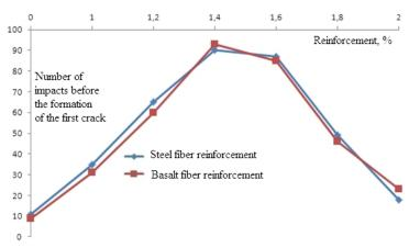
Figure 6. Dependence of the number of strokes before the formation of the first crack on the volume concentration of fiber.
