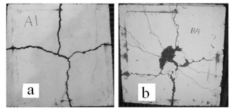
Figure 8. Destruction of samples without fiber and with fiber.
