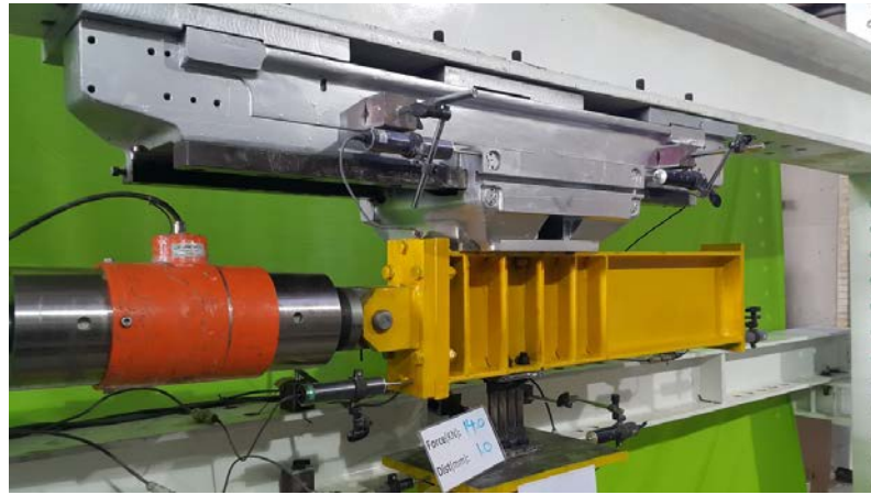
Figure 9. The LMguide and the location of the LVDT units.
