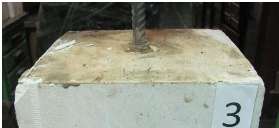
Figure 1. Type of prototype when the anchor displacement is relative to the upper surface of the stone 0.4 mm
