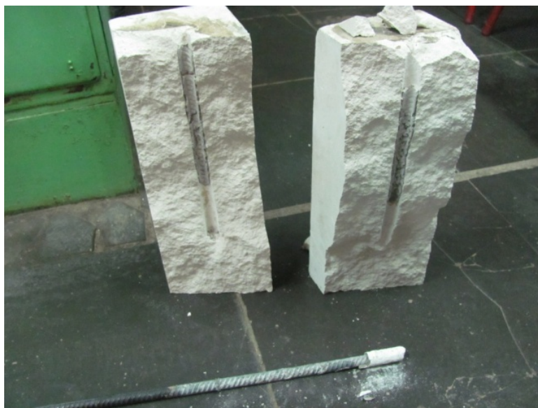
Figure 2. When the anchor was displaced more than 0.4 mm, it was pulled out, followed by a subsequent split of the stones
