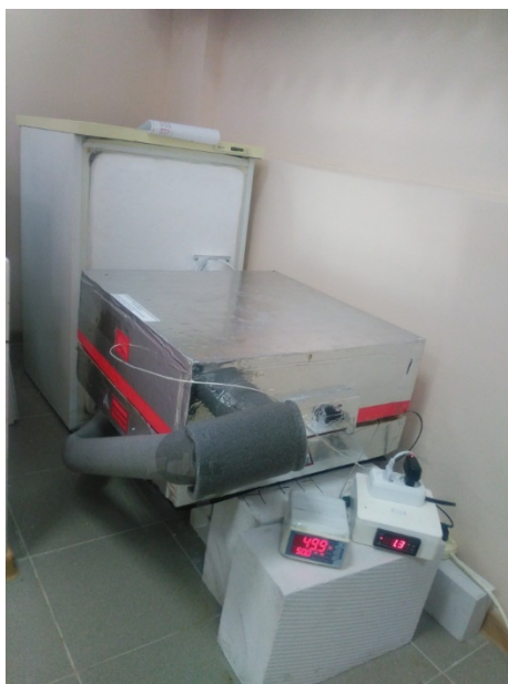
Figure 4. Installation for testing in accordance with GOST EN 12088-2011
