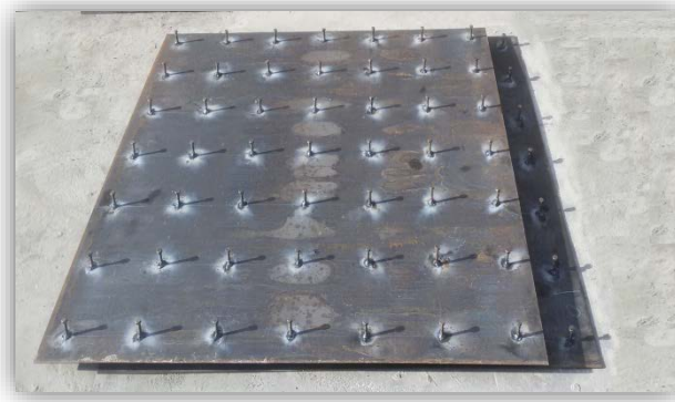
Figure 2. Steel plate with welded stud shear connectors.
