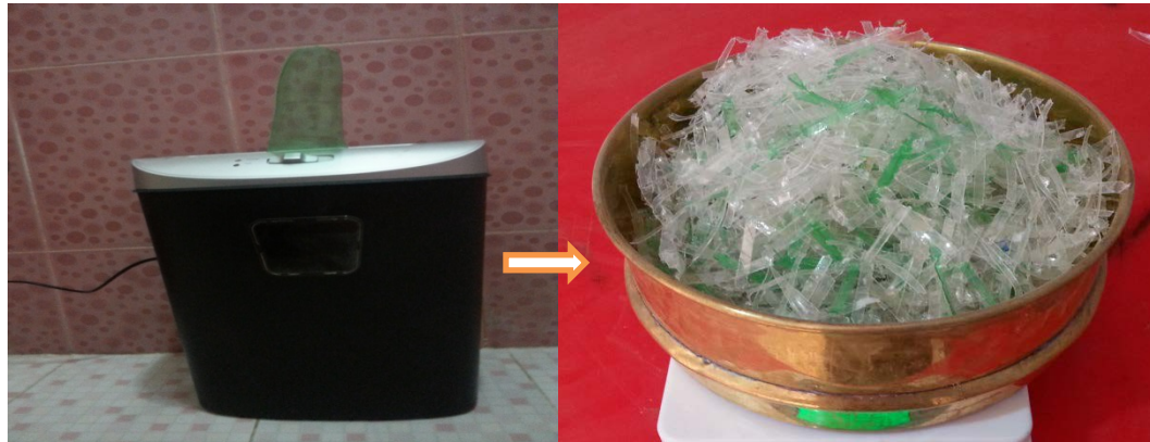
Figure 1. Preparation of plastic fibers: shredding machine(left), and plastic fibers(right).
