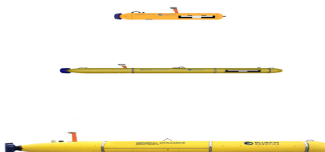
Fig. 2. Example of BLUEFIN-9, BLUEFIN-12 and BLUEFIN-21 AUVs
