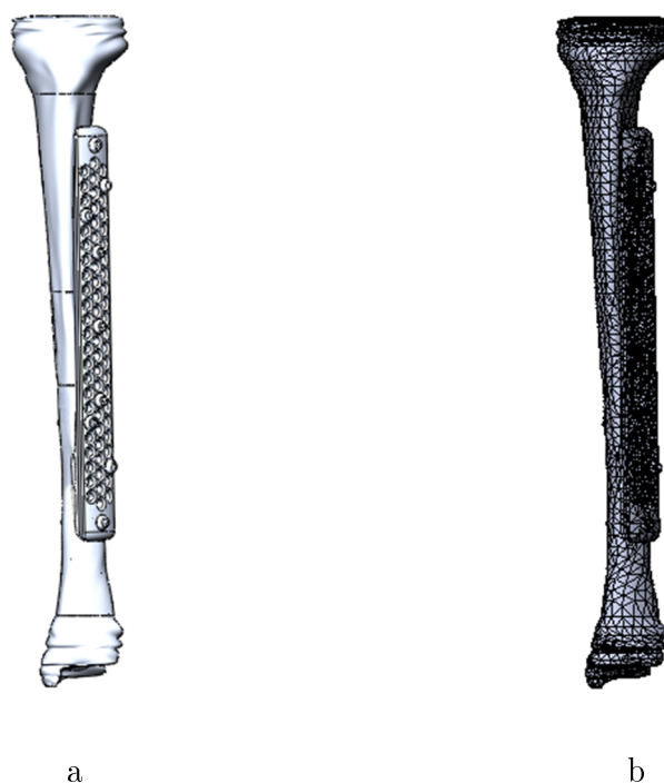
Figure 1. BTS "tibia bone–TRKh plate–screws": a — 3D computer model, b — 3D computer finite element model
