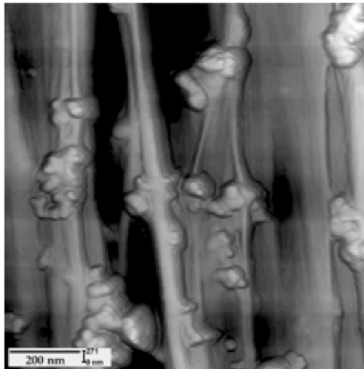
Figure 1: Stretched high-strength bonds between aggregates of carbon black particles obtained by atomic force microscopy
