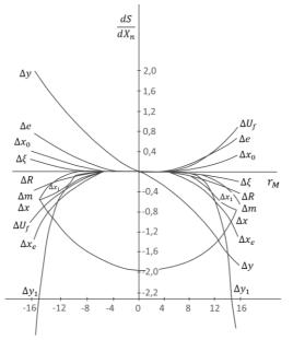
Fig. 3: The curves of phase deviation on the antenna aperture plane.
