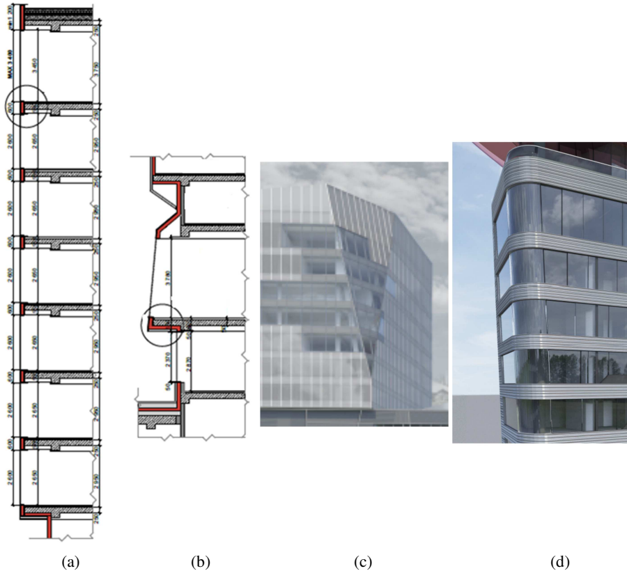
Fig. 1. The geometry of façades for the considered fire scenarios. (a) scenario-1; (b) scenario-2; (c) scenario-3; (d) scenario-4.
