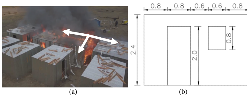
Fig. 1. (a) Flame spread between dwellings (Taken from the IRIS-Fire large scale test, May 2018) (Photo credits: Rodney) and (b) Dwelling front wall design.
