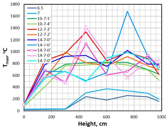
**Fig. 8.** Distribution of maximum combustion temperature for stratified and uniform hydrogen-air mixtures.
