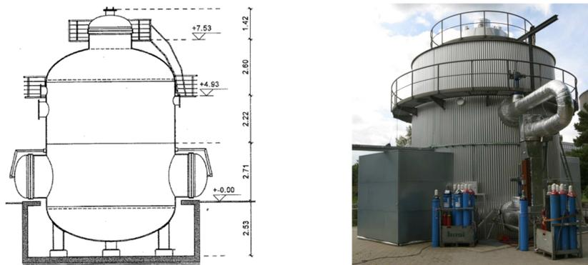
Fig. 4. HYKA-A2 facility: main dimensions and a side view.
