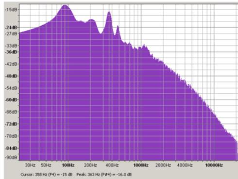
**Fig. 12.** Spectrum of sound record for stratified combustion of the mixture with a gradient 12-7-2%  $H_2$ .
