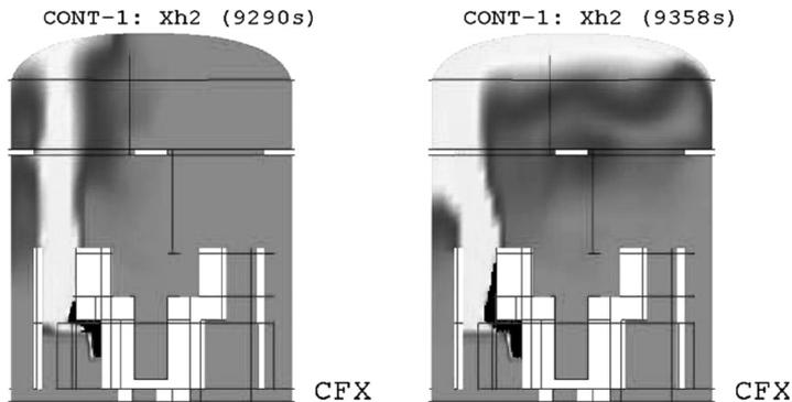
**Fig. 2.** Hydrogen distribution at a vertical plane through the break room of the PWR Westinghouse case [5].
