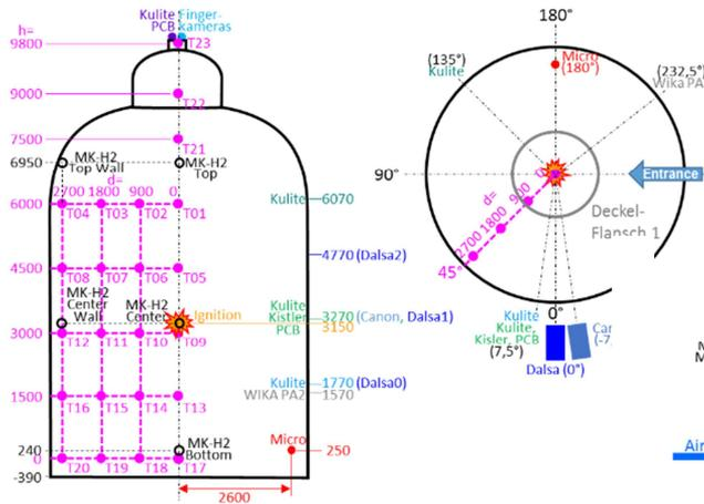
**Fig. 5.** Positions and orientation of sensors: thermocouples (T); gas analyzer (MK-H2); microphone (Micro). A center ignition position (CI) is shown.
