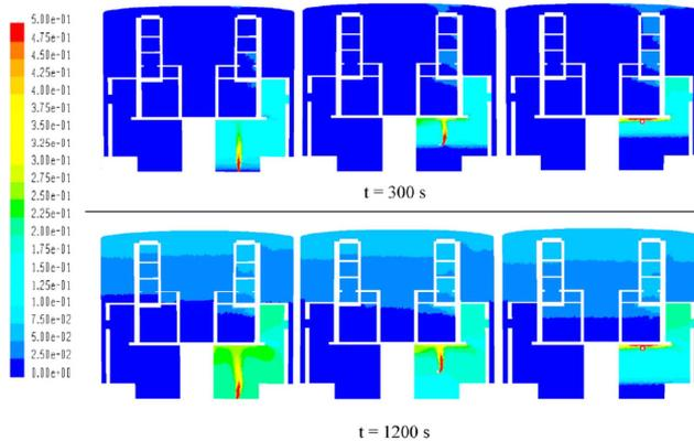
**Fig. 1.** Distribution of hydrogen for different injection time [4].
