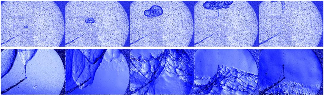
**Fig. 13.** A sequence of BOS images for non-uniform combustion with a gradient 10-7-4%  $H_2$ .
