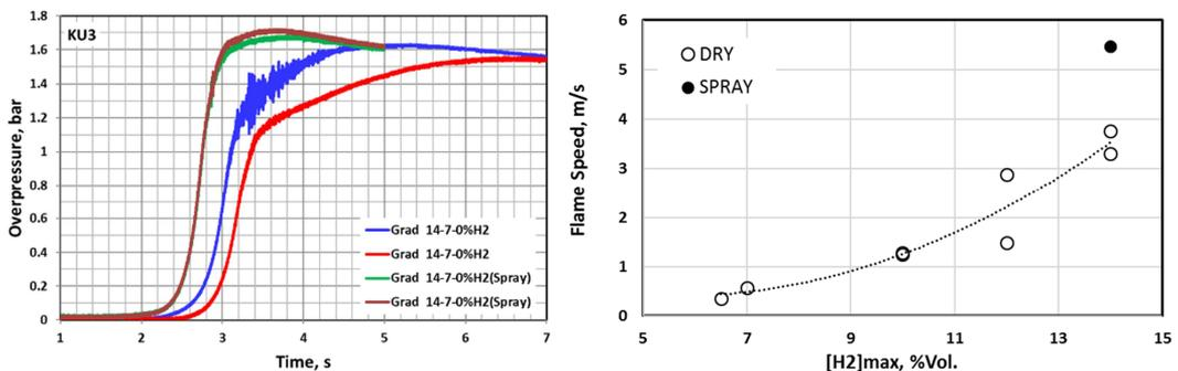
**Fig. 11.** Maximum combustion pressure (left) and visible flame velocity as function of maximum hydrogen concentration (right) for dry mixture and wet composition in presence of water spray.
