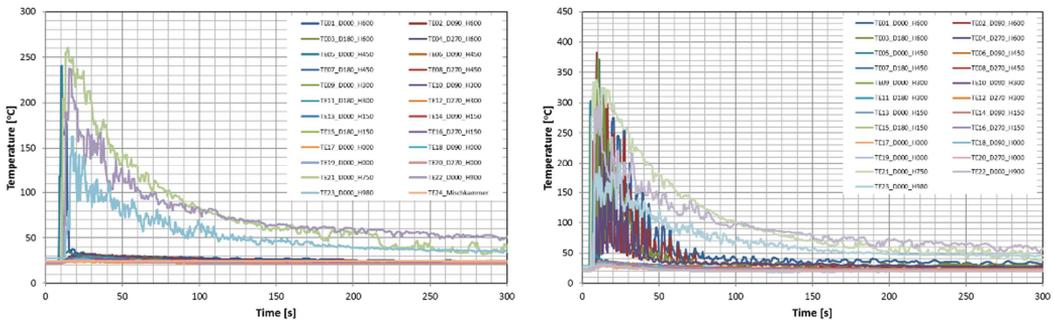
**Fig. 9.** Maximum combustion temperature for uniform compositions of hydrogen – air mixtures with 6.5% (left) and 7% H<sub>2</sub> (right).
