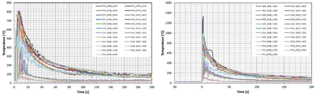
**Fig. 10.** Maximum combustion temperature for stratified compositions of hydrogen-air mixtures with two gradients from 10=>7=>4% H<sub>2</sub> (left) to 12=>7=>2% H<sub>2</sub> (right).
