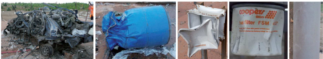
Fig. 6. Damage to some of the items placed inside a propane detonation [41]. Damage created by overpressure > 10 bar. Note the dark markings on the post (extreme right) facing opposite to detonation propagation.
