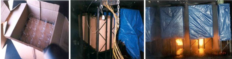
Fig. 13. Scaled MSC 914 tests: cartons, configuration, and suppression of fire.
