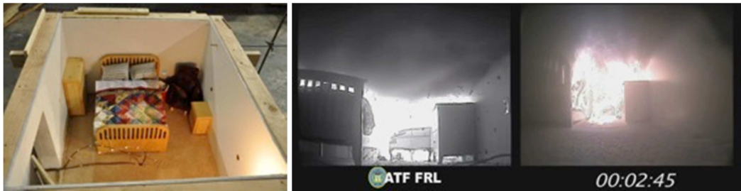
Fig. 16. Scale modeling of a bedroom fire.
