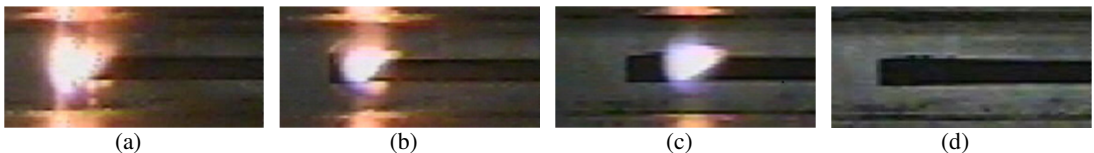
Fig. 5. Combustion and self-extinction of an element from fiberglass plastic in zero-gravity under gas flow rate velocity of 20 cm/s, and oxygen concentration of 23.0 %.
