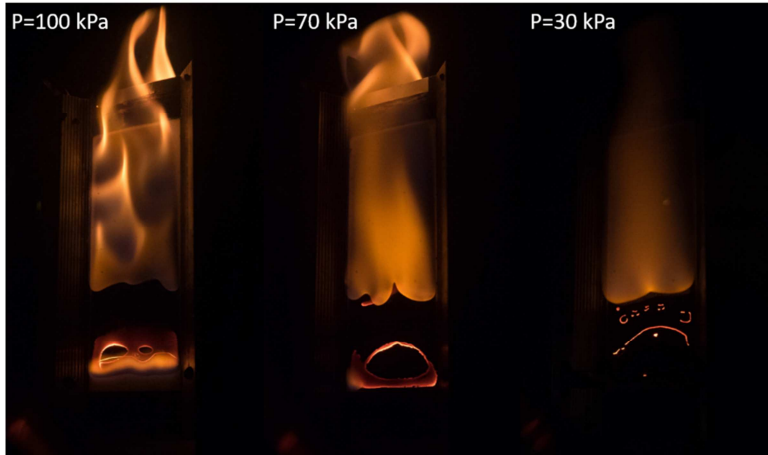
Fig. 7. Visible flame as a function of ambient pressure.
