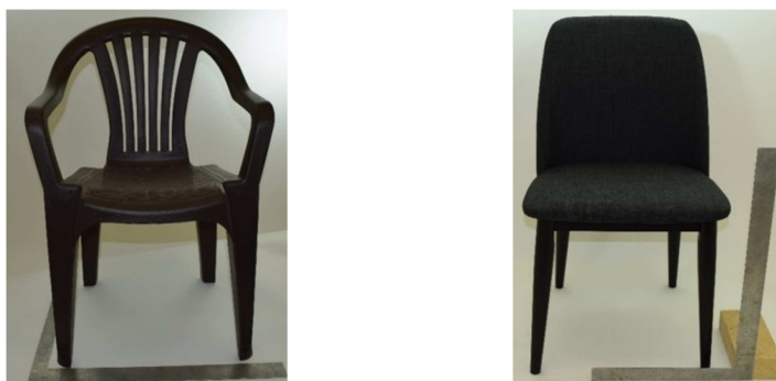
Fig. 1. Pre-test photographs of the polypropylene (left) and wood/foam/fabric chairs (right).
