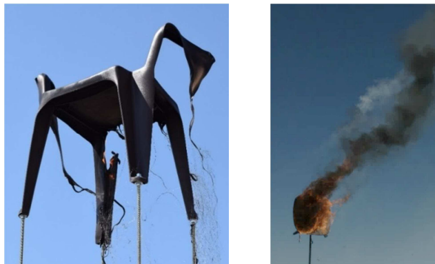
Fig. 7. Post-exposure flaming of the polypropylene chair (left) and the fabric chair (right).
