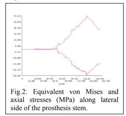
The largest stresses equal to 76.6 MPa were obtained for the third gait phase, especially around the lateral part of the prosthesis under the spigot (Fig.2). We especially noticed that stress redistribution is around the prosthesis. A higher stiffness of this implant is responsible for the lack of stresses in the other parts of the bone.
