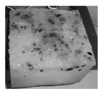
Figure 1. Oil included in the ice slush. Sample of oil in ice slush frozen together
