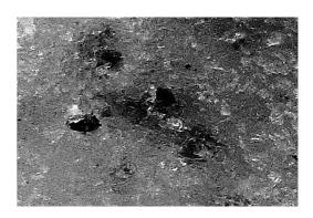
Figure 2. Holes on the top of ice due to oil drops
