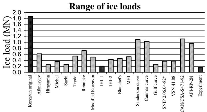
Figure 1. Correlation between ice loads obtained from experiment and value of ice load calculated with different methods
