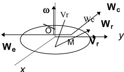
$$\begin{aligned} w_{ry} &= y^{**} = 6 \\ w_e &= w_e^{oc} = \omega^2 OM = 4 \text{ м/сек}^2 \\ w_c &= 2\omega v_r = 16 \text{ м/сек}^2 \end{aligned}$$
