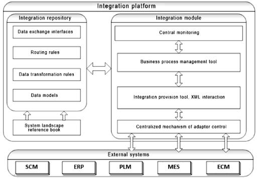
Fig. 4. Integration bus architecture
