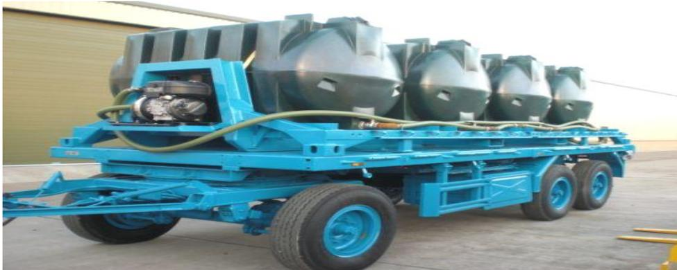
*Fig 4. Automatic fuel tanker on Thompson trailer chassis*
