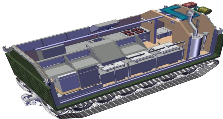
*Fig. 3. The technological kitchen block Arctic Ka-250/r*
