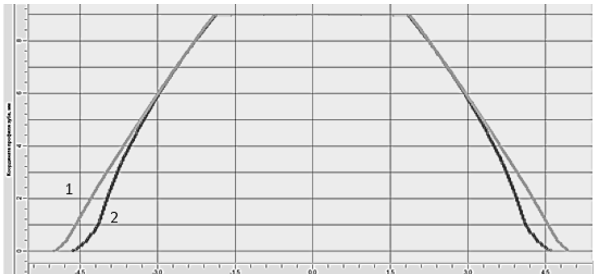
Figure 3 –Tooth profile: 1 – pinion tooth shape, 2 – gear wheel shape
