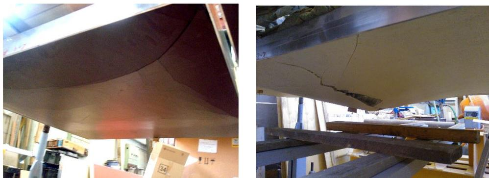
**Figure 11. Destruction of cassette under the influence of distributed load**
