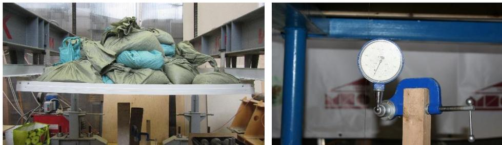
**Figure 6. Testing stand (left) and deflectometer 6PAO (right)**
