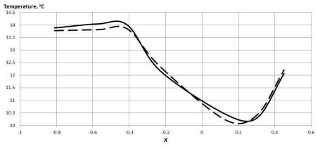
Figure 4. Values of the minimum temperature τ<sub>slope</sub> by changing the window block position
