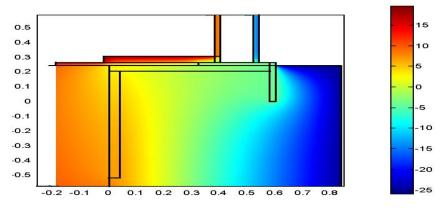
Figure 2. Temperature field of the side section of the window slope
