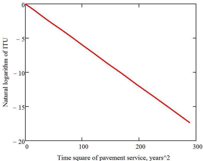
**Figure 9. Linearized dependence of ITU on time square**
