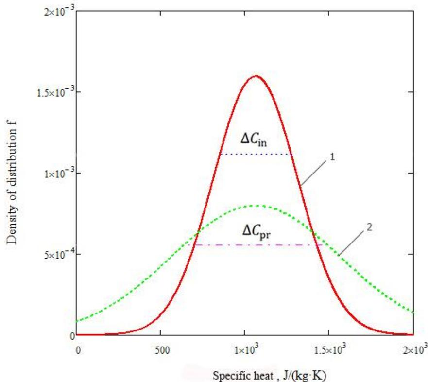
**Figure 7. Normal distribution of specific heat C (density of distribution f):**
