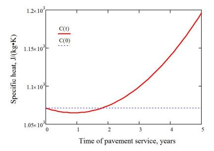
Figure 3. Dependence of the asphalt concrete specific heat versus time
